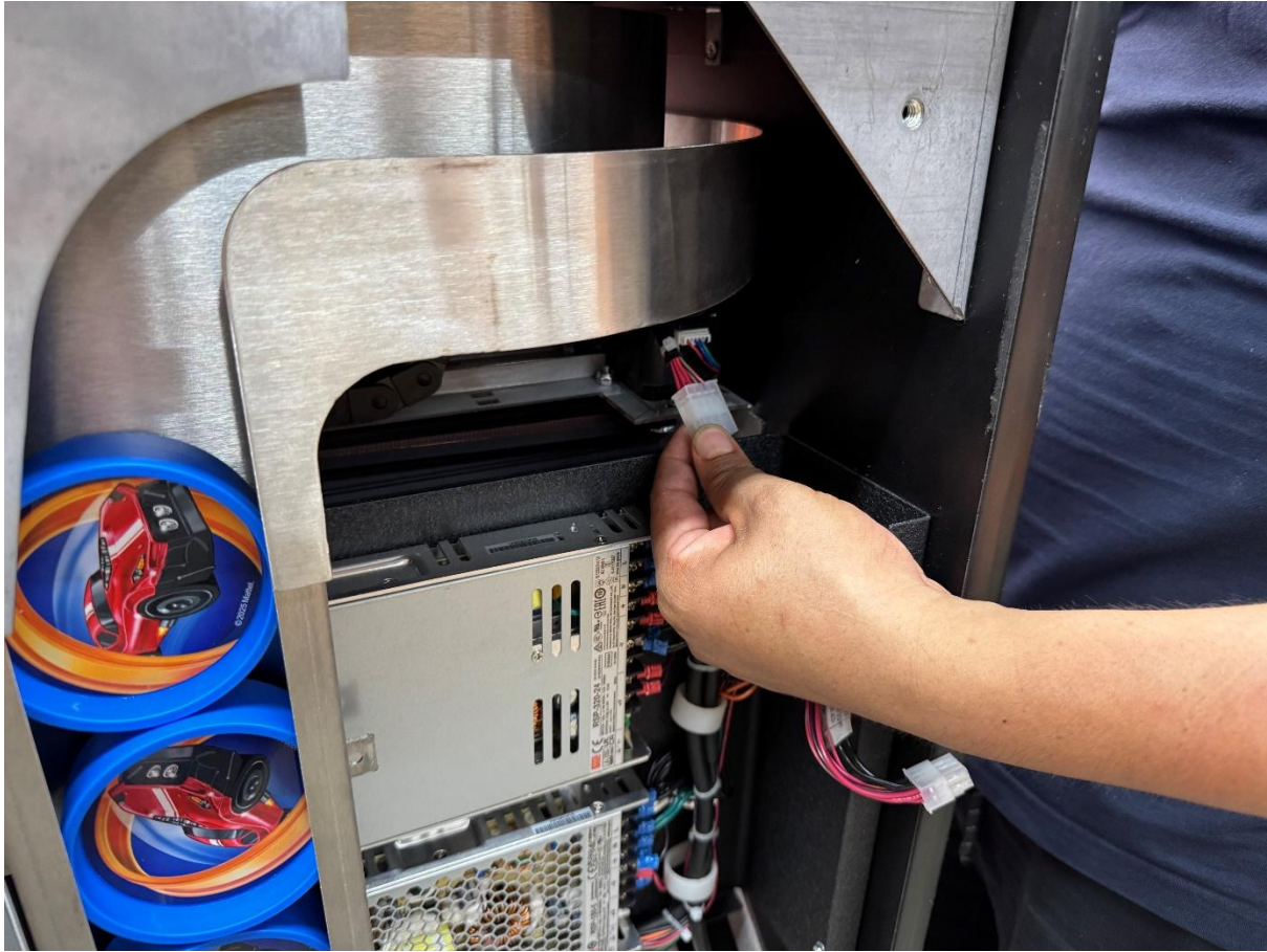
Connect puck track harness. Dress cable to prevent interference with travel of displays.
