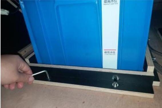
Step 1: Remove the screws of tank baffle.
