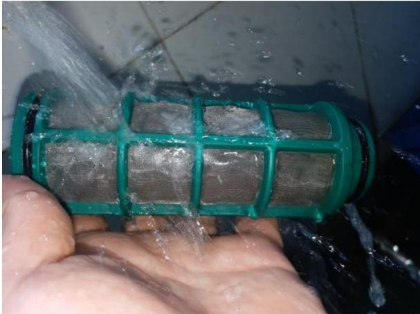
Step 7: Remove the filter element and rinse with tap water until the dirt is flushed.
