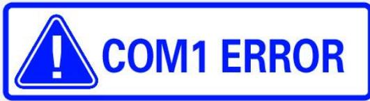
2. **Cause: No enough tickets, or the ticket machine is damaged**
